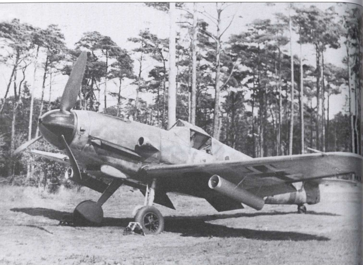
Bf 109G-2 of JG 11 based at Jever late in 1943, fitted with underwing launchers for two 21-cm air-to-air rockets for use against US heavy bomber formations.
