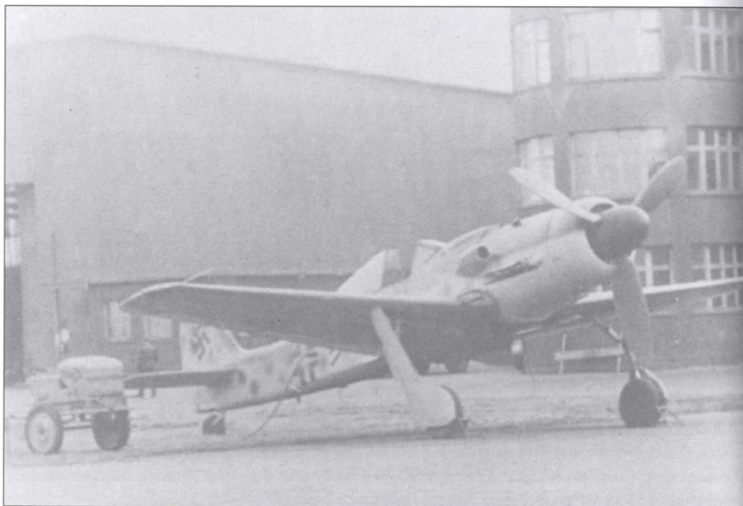
The Focke Wulf Fw 190D entered service in the summer of 1944. This sub-type of the famous fighter was fitted with the Jumo 213 in-line engine, resulting in lengthened nose contours. The performance of the Fw 190D was similar to that of the best Allied fighters of the late war period.
