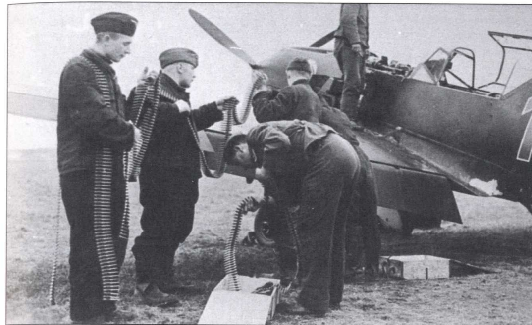
Ground crewmen reloading the wing and engine-mounted 7.9 mm machine-guns of a Bf 109C of IIIrd Gruppe of Jagdgeschwader 51 (III./JG 51). Scrupulous cleanliness was necessary for this operation, since any grit or dirt adhering to the rounds might cause a stoppage during firing.
