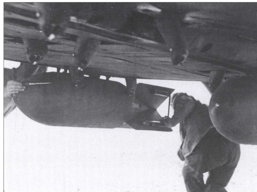
Armourers carry out final adjustments on a 550-pound bomb mounted under the fuselage of a He 111. Note the compressed cardboard 'screamers' fitted to the fins of the bomb, intended to increase the weapon's effect on enemy morale.
