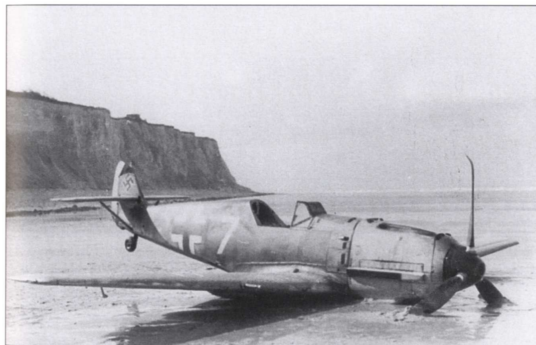
During the daylight attacks on London the escorting Bf 109s had to operate at the limit of their radius of action. Several of these fighters were lost when they ran out of fuel, and this one only just made it back to the coast of France. via Willis
