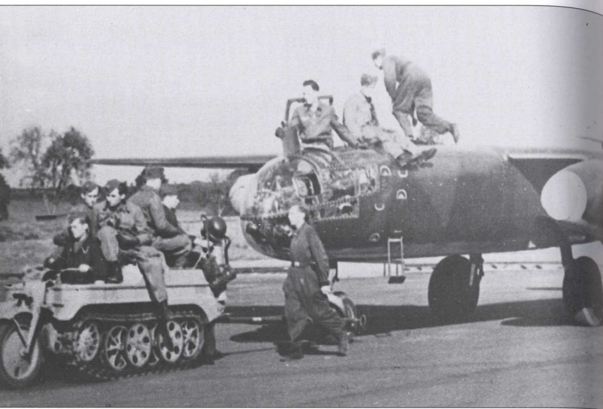
Kettenrad tractor used to tow an Ar 234 back to its dispersal after a flight.
