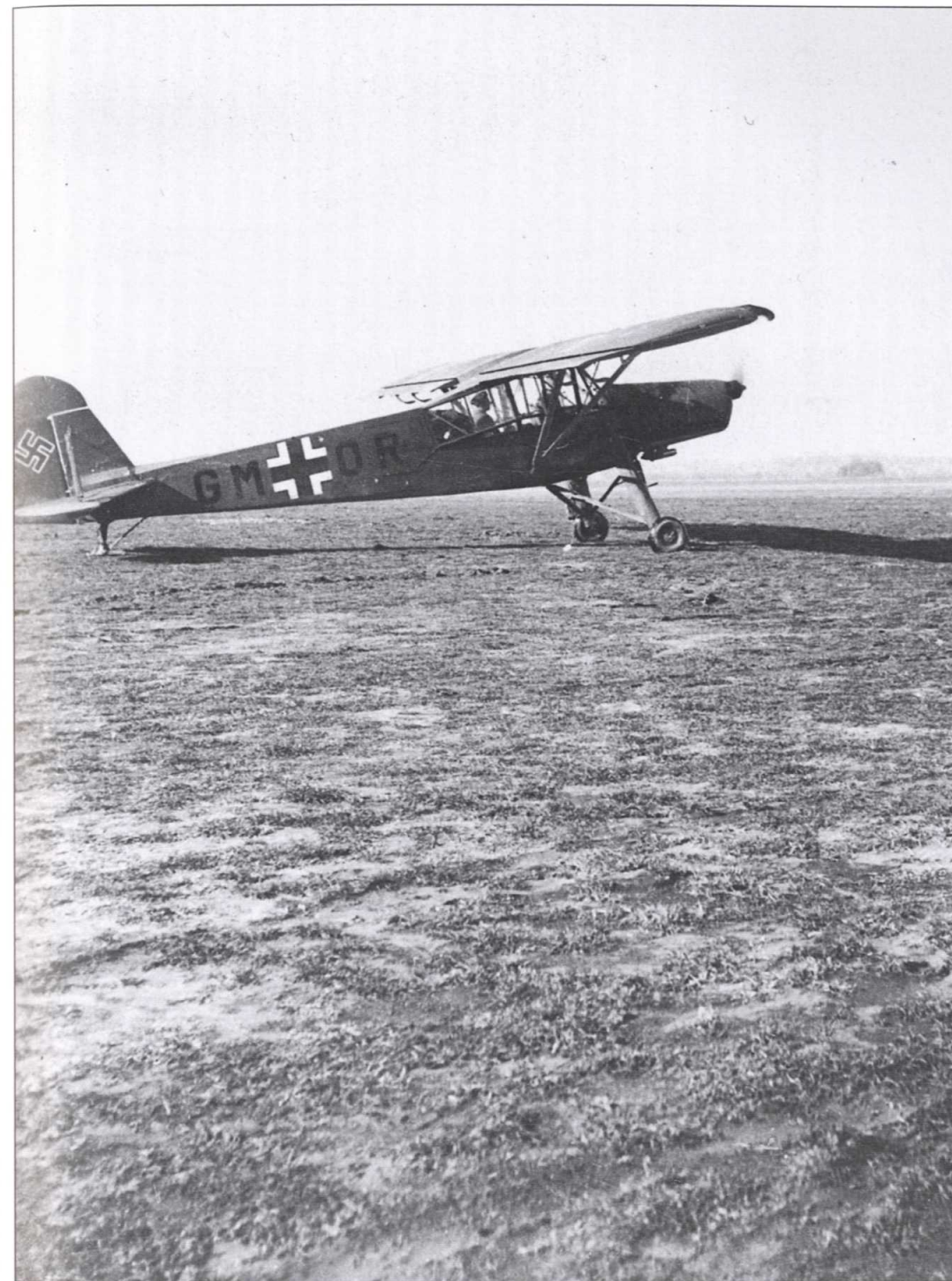
The Fiesler Fi 156 Storch, with an outstanding short take-off and landing capability, was used in large numbers on the Eastern Front as a light transport and liaison aircraft.
