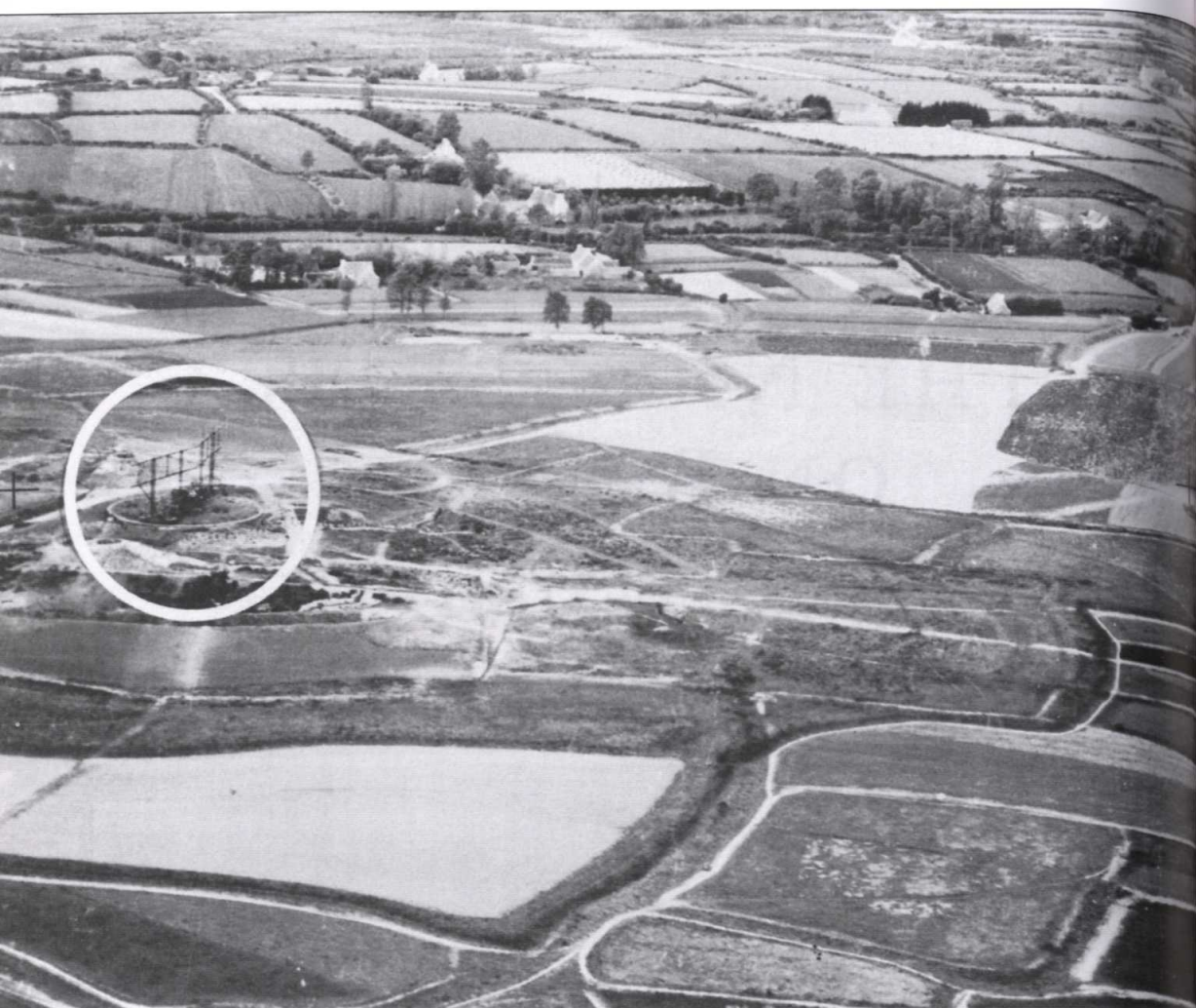
'Knickerbein' transmitting station situated at Mount Pinçon, near Saint Lô in northern France. The station radiated a narrow radio beam at high power, which was accurately aligned on the target to be attacked. The beam signals were picked up by the standard airfield approach receivers carried by all German bombers, and no special equipment was necessary for crews to use this system.
