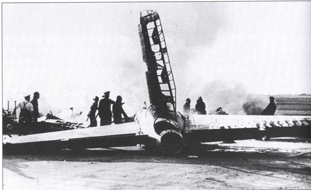
The coupled engine arrangement on the He 177 gave constant trouble, however, and several of these bombers were lost following engine fires. A premature attempt to introduce the aircraft into service in 1942 ended in failure, and after several aircraft were destroyed in accidents the type had to be withdrawn for modification. via Schliephake
