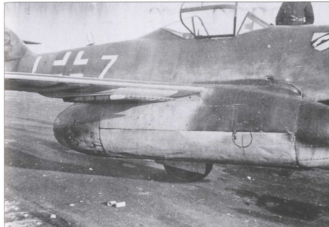
Me 262 of Jagdgeschwader 7, with a rack for twelve 55-mm air-to-air rockets mounted under each wing. First used in action in March 1945, these unguided weapons were ripple-fired in one burst at a single target.
