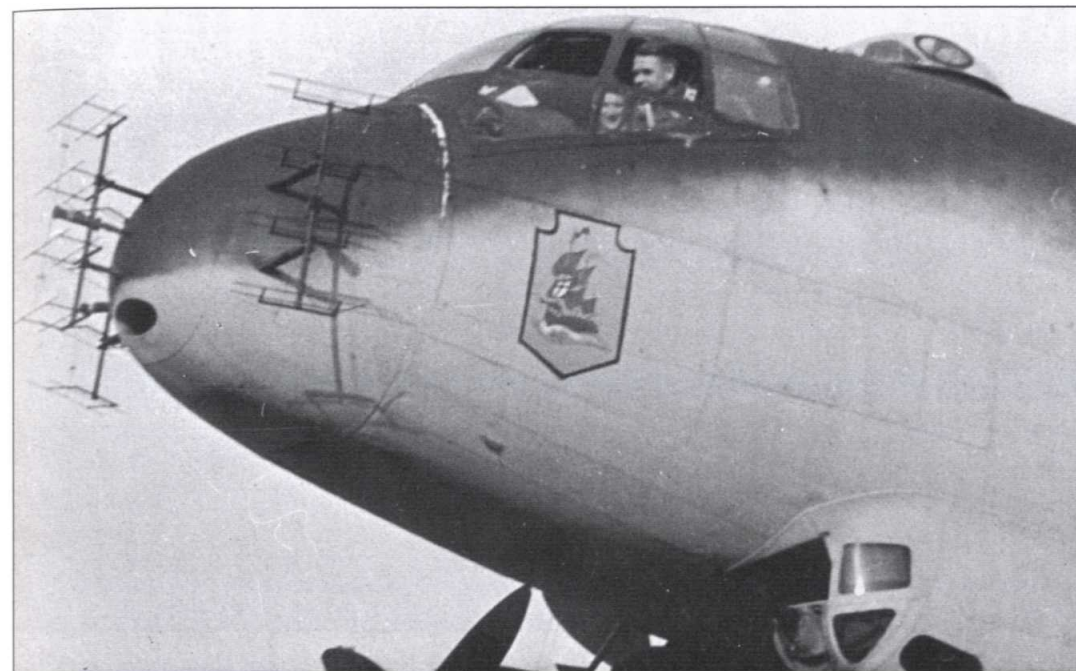
Radar-fitted Junkers Ju 290 long-range reconnaissance aircraft flown by Fernaufklärungsgruppe 5 (FAG 5) operating from Mont de Marsan in south-west France. This unit flew reconnaissance missions far into the Atlantic, searching for convoys for U-boats to attack. via Obert
