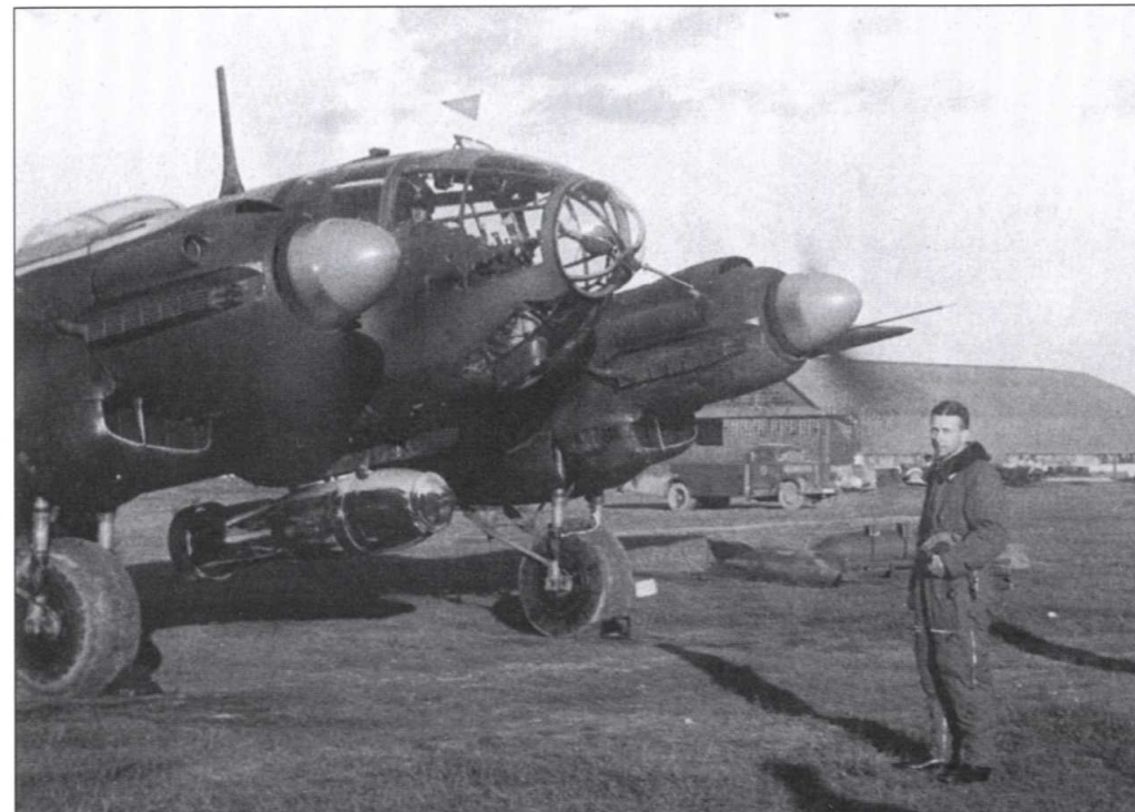
He 111 of III./KG 26, a night-attack unit that employed the Y-Gerät beam bombing system (note the additional aerial aft of the cockpit). This device proved no more successful than the X-Gerät during attacks on targets in Great Britain, however. The man in front of the aircraft (above) and in the cockpit (below) is Major Viktor von Lossberg, the Gruppe commander. von Lossberg
