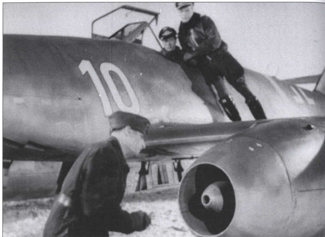
Ground crewman pulls the lanyard to start the small two-stroke piston engine built in the nose cone of the jet engine. The piston engine served as the starter motor for the Jumo 004 turbojet.
