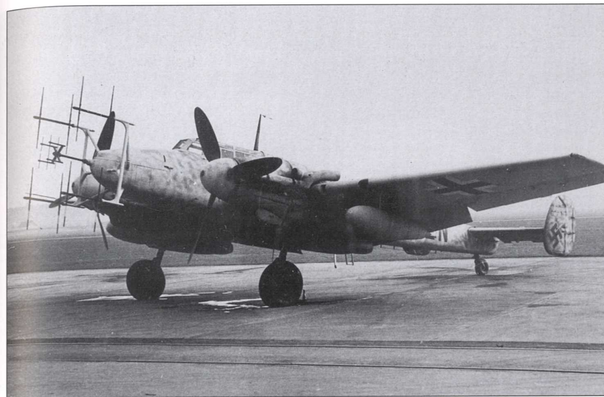
Bf 110G pictured early in 1944, with the large aerial array for the new SN-2 radar and a smaller array for the separate FuG 212 radar in the centre.
