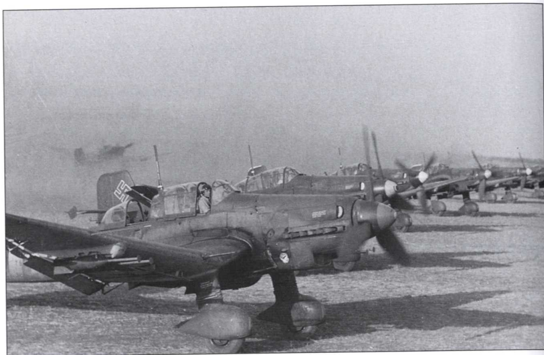
Junkers Ju 87D dive-bombers of 1./StG 2 about to take off for a mission over Russia. At the controls of the leading aircraft was the dive-bomber ace Oberleutnant Hans-Ulrich Rudel. Note the fuse extensions fitted to the bombs on the underwing racks, to detonate the weapons just above ground level.
