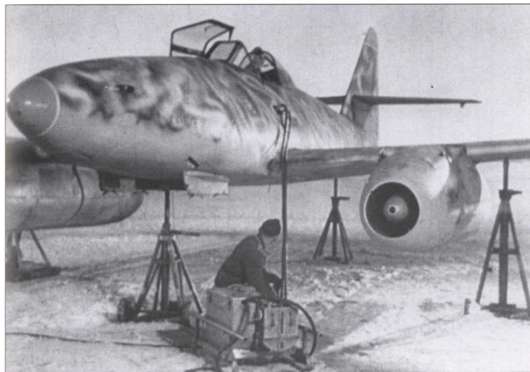
The two-cannon armament and bomb racks under the nose identify these aircraft as a Me 262 fighter-bombers of Kampfgeschwader 51. The aircraft on jacks is having the undercarriage retraction system tested.
