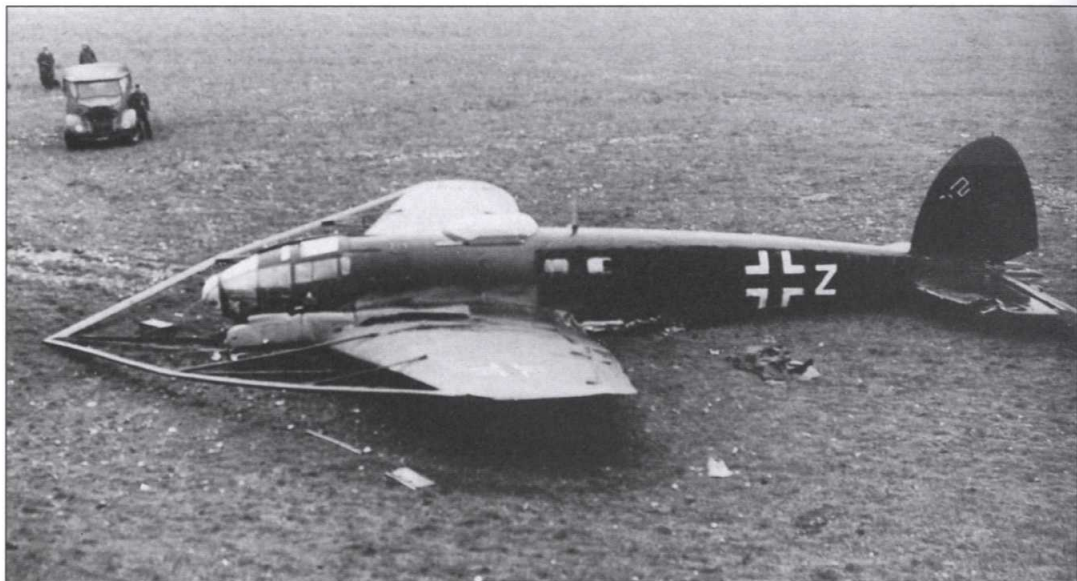
This He 111-8 from IL/KG 27 was running in to deliver a low-altitude night attack on Yeovil when it struck a mist-covered hill near Lulworth Cove, 22 May 1941. The bomber carried a fender attachment mounted in front of the nose and wings to ward off barrage balloon cables. The fender weighed about 550 pounds and required a similar weight of lead in the rear fuselage to serve as a counter-balance. The additional weight and drag of the installation reduced the performance of the aircraft and impaired handling. The device was unpopular with crews, and after a short time it was removed from front-line aircraft.
