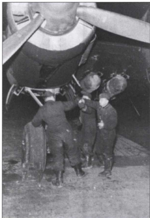
Ground crewmen of KG 1 crank the inertia starter handle to start the starboard engine of a Ju 88 of KG 1, before a night attack on Great Britain.
