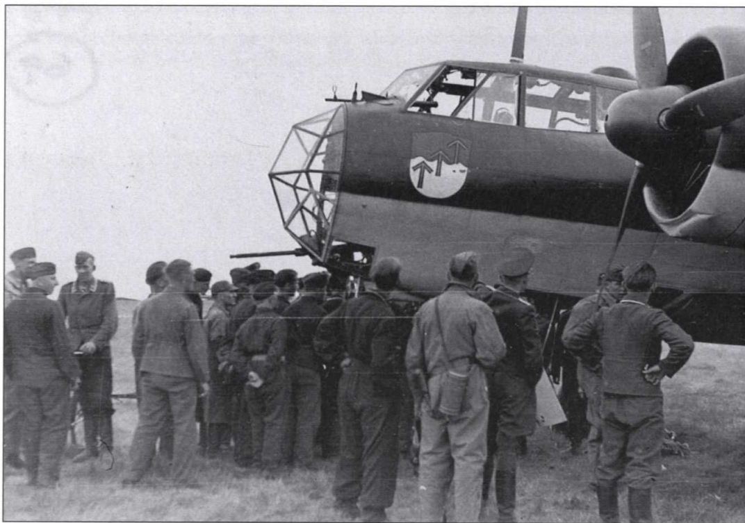
Do 17 of IIInd Gruppe of KG 76, fitted with 20 mm cannon in the nose for strafing ground targets. Raab
