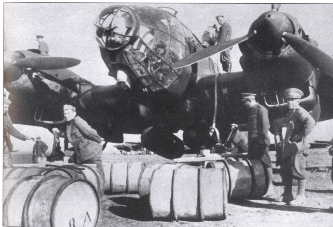
Italian airmen at the airfield on Rhodes assist with the refuelling of an He 111 of KG 4. Beneath the bomber are two LMB 1,000-kg magnetic mines, probably intended for the approaches to Alexandria harbour or the Suez Canal. via Michulec
