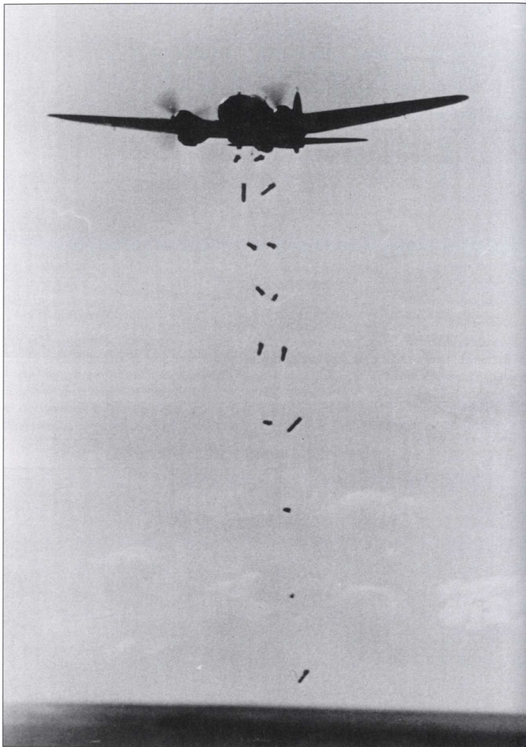
A He 111 releases a string of 110-pound high-explosive bombs. These small weapons were suspended in the bomb bay nose-up, and after release they tumbled into the nose-down position.
