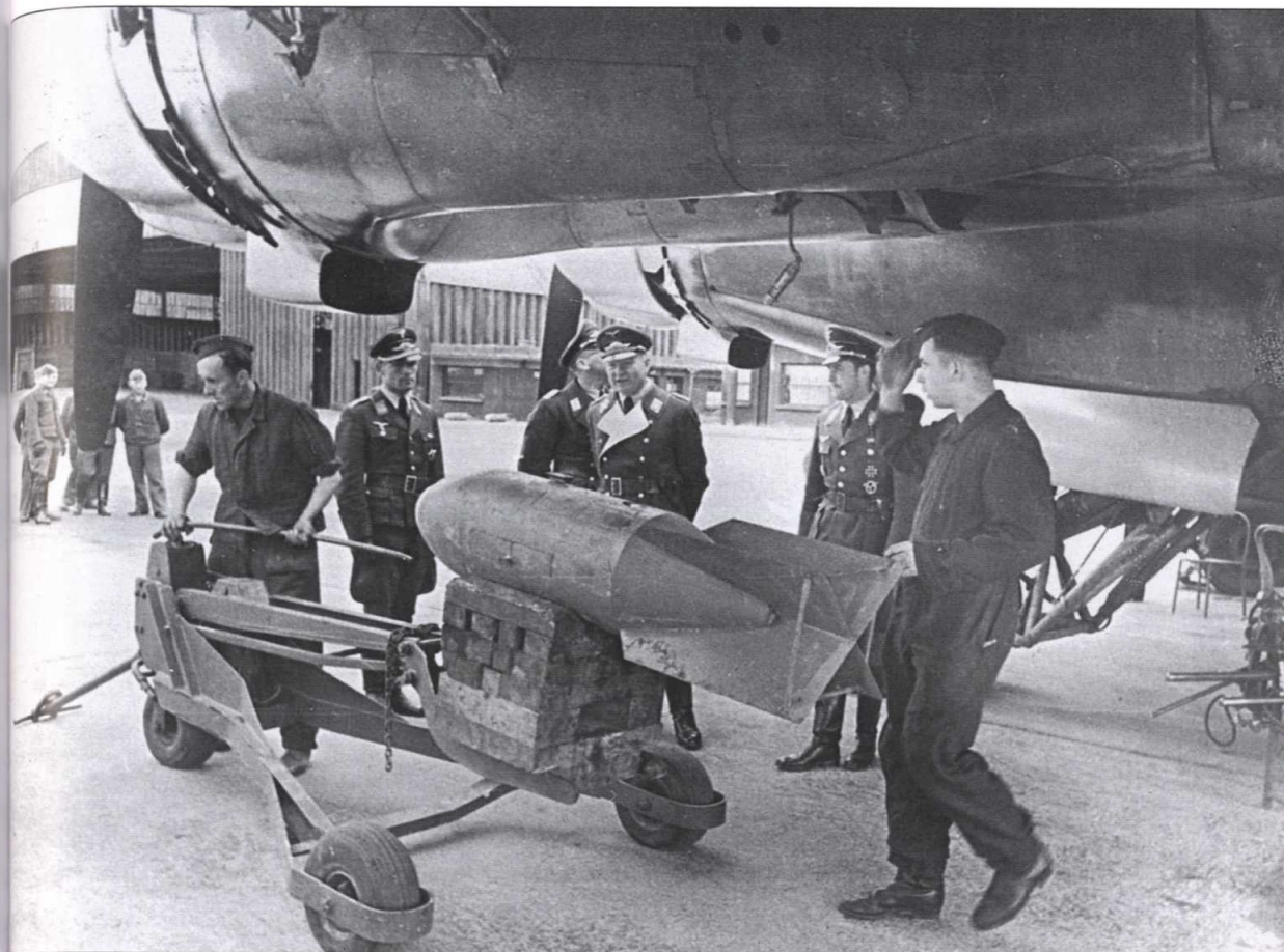
Armourers loading an 250-kg bomb on the rack under the port outer engine of an Fw 200. Joep
