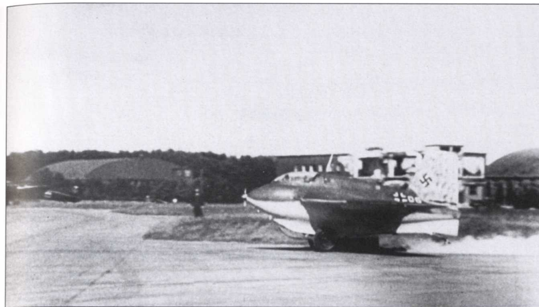
The rocket-propelled Messerschmitt Me 163 fighter was the first jet-propelled aircraft to enter operational service in any nation, in May 1944. Although it had a sparkling turn of speed and excellent climbing performance, the fighter had a pitifully short radius of action and that constrained its military effectiveness. These examples belonged to JG 400, the only combat unit to receive the type. via Ethell
