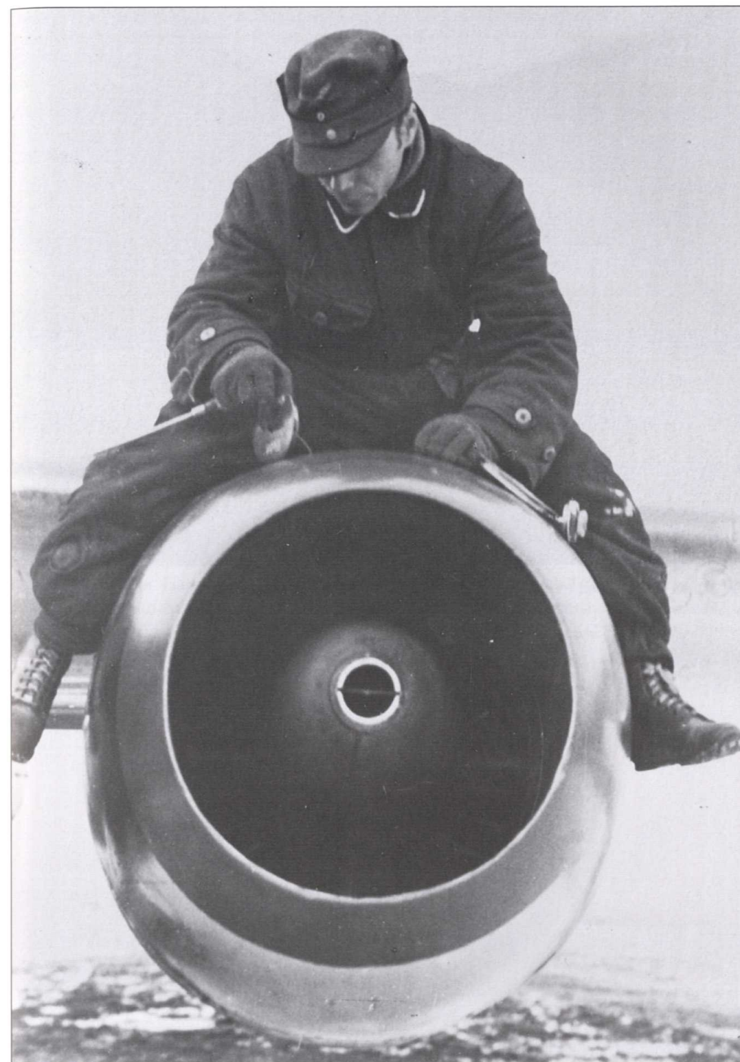
A groundcrewman straddles the Jumo 004 of an Ar 234, to show the small diameter of the turbojet.
