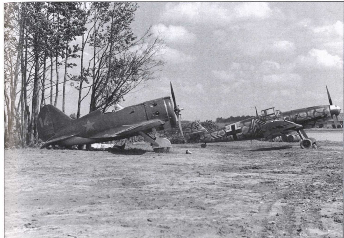
Me 109 'Friedrich' of JG 54 beside a captured Soviet I-16 fighter. The more powerful and cleaner-lined German fighter had a considerable speed advantage over its enemy counterpart, especially at high altitude.
