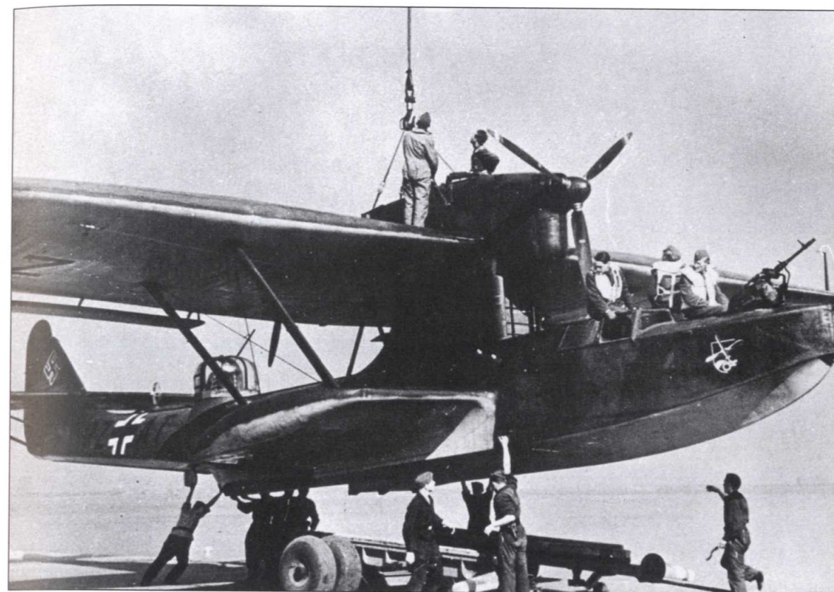
Dornier Do 18G flying boat being lowered on to its beaching trolley. This maritime reconnaissance type was obsolescent at the beginning of the war, and in 1941 most of those remaining were relegated to the air-sea rescue role. via Michulec
