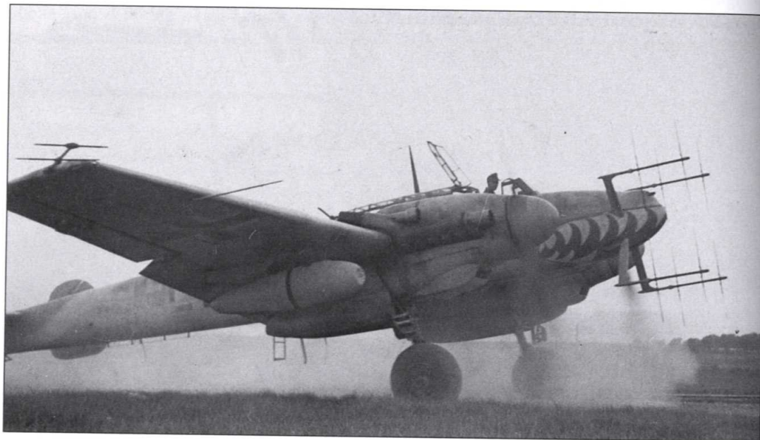
Bf 110Gs fitted with a later version of the SN-2 radar, with which the FuG 212 was no longer required. The aerial on the wing tip of one of the aircraft fed the 'Flensburg' homing system, enabling the night-fighter to home in on the emissions from the 'Monica' tail warning radar carried by RAF bombers.
