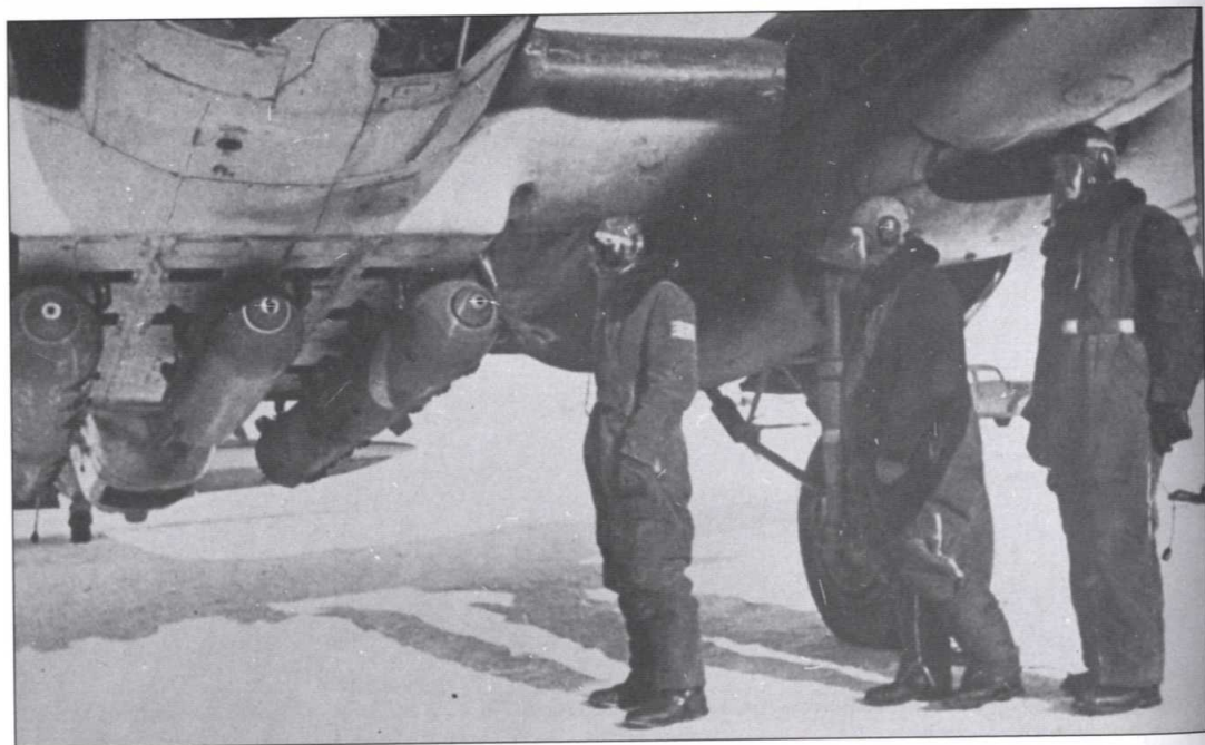
Supply containers mounted on the underfuselage racks of a He 111.
