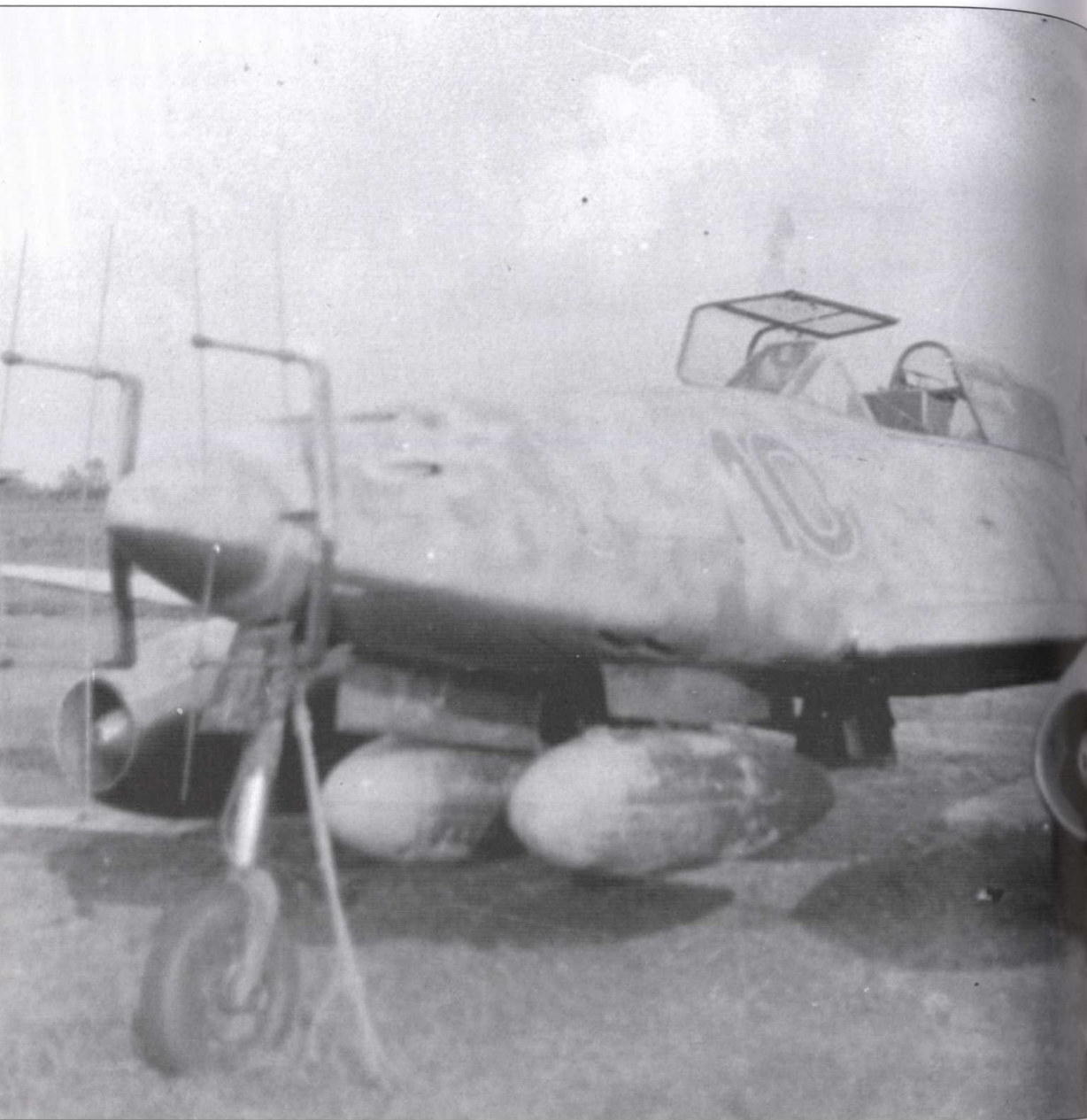
A small number of Me 262 jet fighters were converted for the night-fighter role by the installation of Neptun radar.
