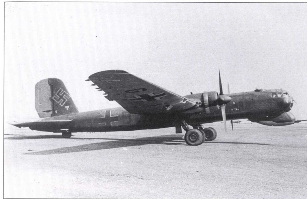
Heinkel He 177 experimentally fitted with a 7.5-cm gun, intended for operations against ground targets on the Eastern Front. The combination was not a success, however, and it was not used in action.
