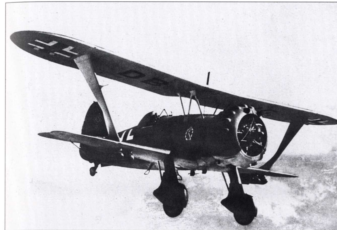
A Henschel Hs 123 ground attack aircraft. Despite its outdated appearance, this type proved effective for strafing ground targets and providing close air support for German troops during the campaign in Poland. via Schliephake
