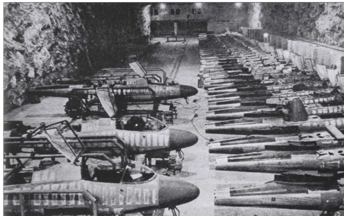
Underground production of He 162 fuselages, in a disused salt mine at Tarthun near Magdeburg.
