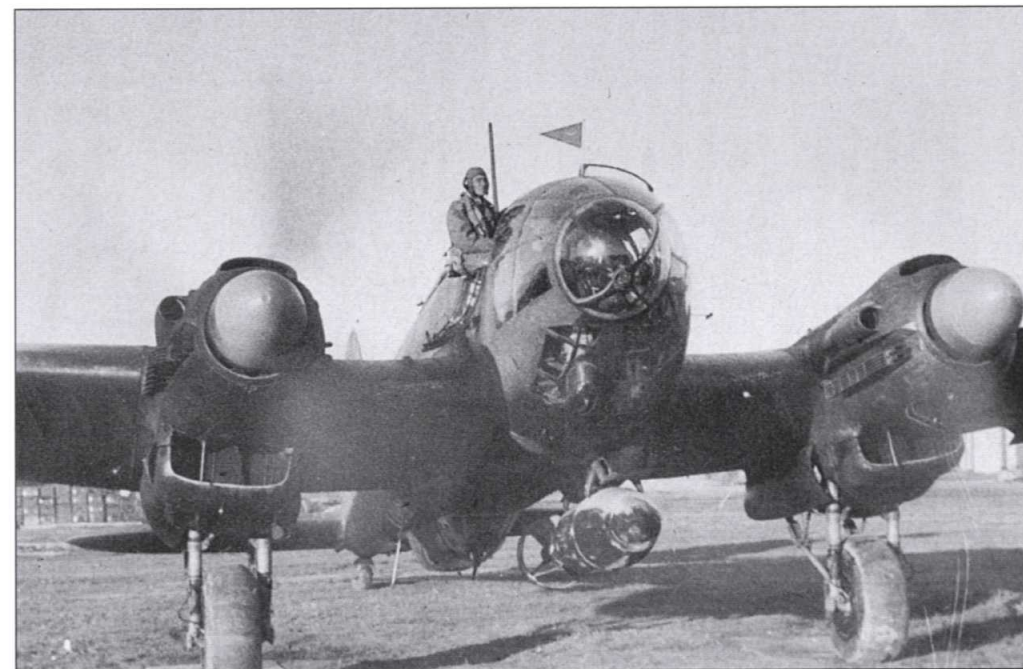
He 111 of III./KG 26, a night-attack unit that employed the Y-Gerät beam bombing system (note the additional aerial aft of the cockpit). This device proved no more successful than the X-Gerät during attacks on targets in Great Britain, however. The man in front of the aircraft (above) and in the cockpit (below) is Major Viktor von Lossberg, the Gruppe commander. von Lossberg
