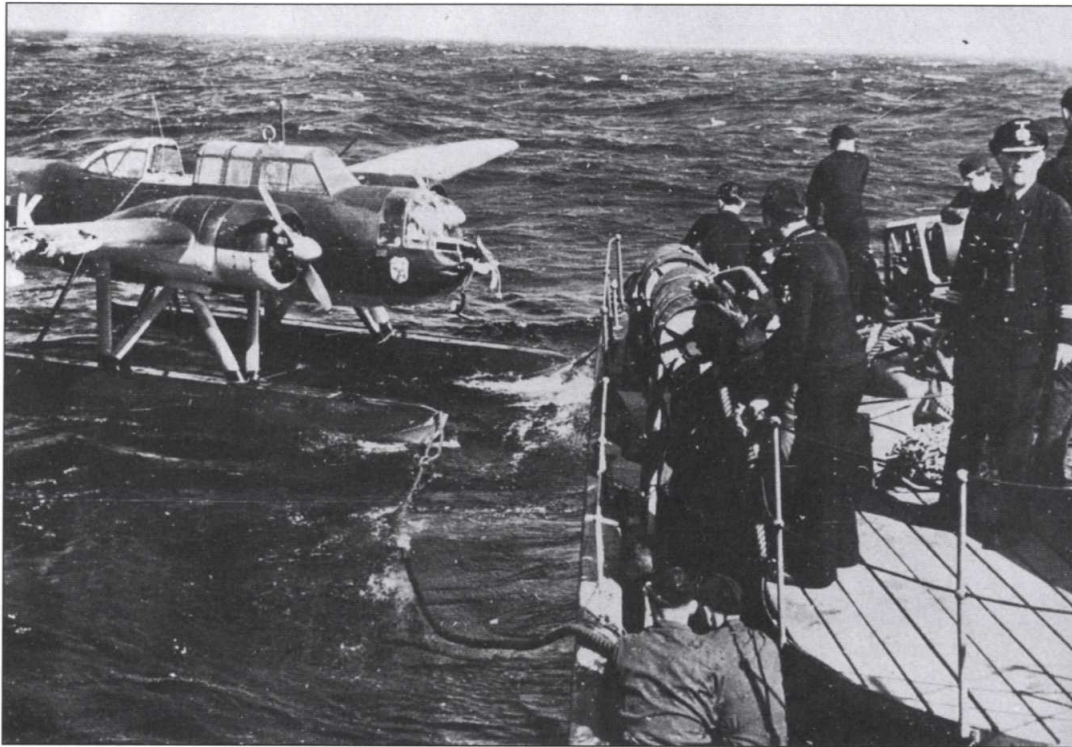
Several types of captured seaplane were pressed into service in the Luftwaffe. This Dutch-built Fokker T VIII of Seeaufklärungsgruppe 126 was being towed by a German warship. This was a difficult operation, however, and the aircraft suffered severe damage to the nose and starboard wing after striking the ship. via Michulec
